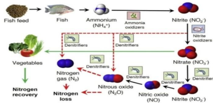
Figure 17 Nitrogen transformations in aquaponics systems (Wongkiew et al. 2020).
