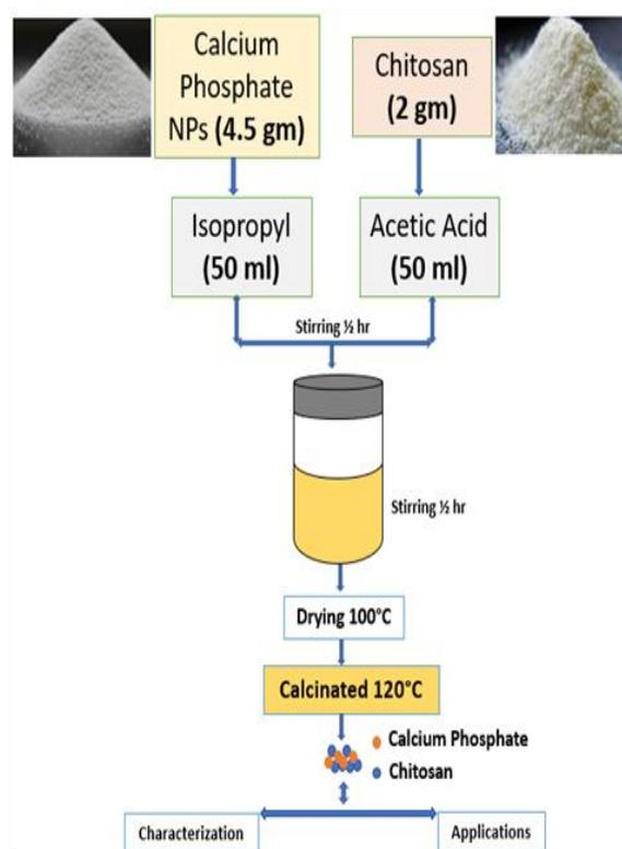
Figure 1 Schematic illustration of CaP-CS NC preparation
