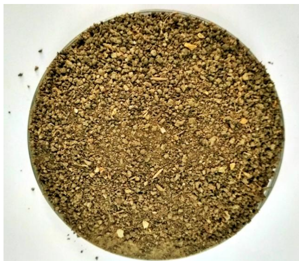
Figure 1 Experimental material sewage sludge collected from Bhagwanpur Sewage Treatment Plants (STPs) after dry
