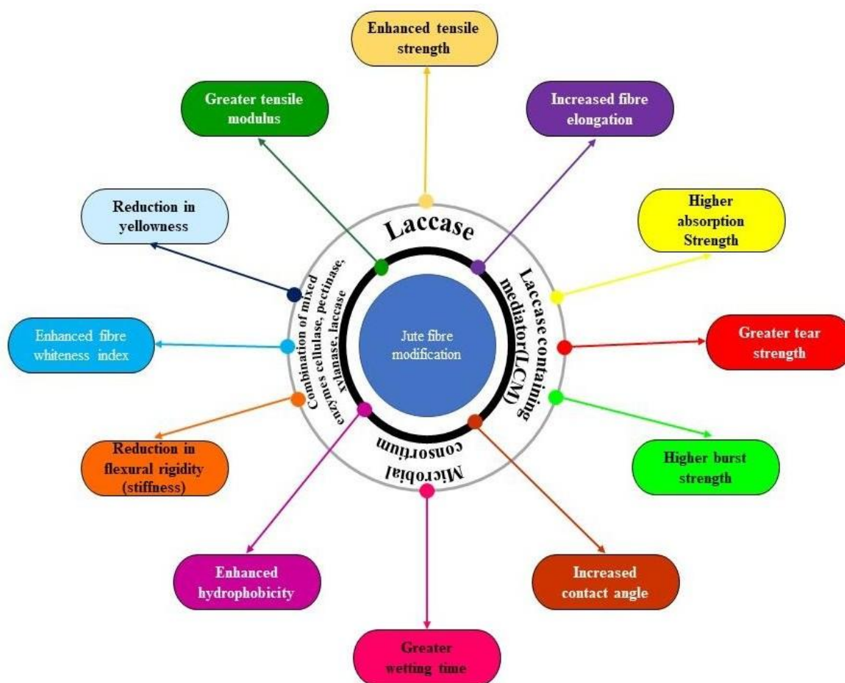
Figure 2 Jute fiber modification by laccase and combination of mixed enzymes (cellulase, pectinase, xylanase, and laccase)
