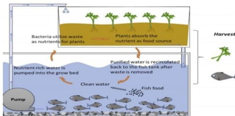
Figure 3 Schematic diagram of Aquaponics (Wei et al. 2019)
