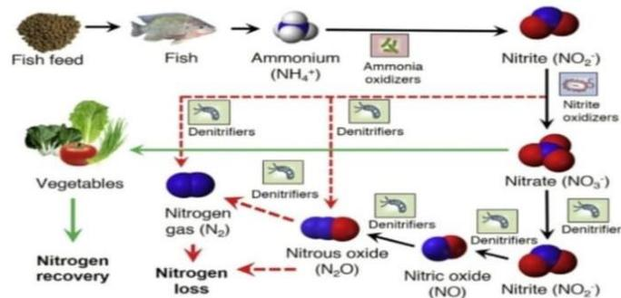
Figure 17 Nitrogen transformations in aquaponics systems (Wongkiew et al. 2020).
