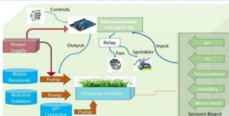
Figure 8 Fully Automated hydroponics system (Shetty et al. 2021).
