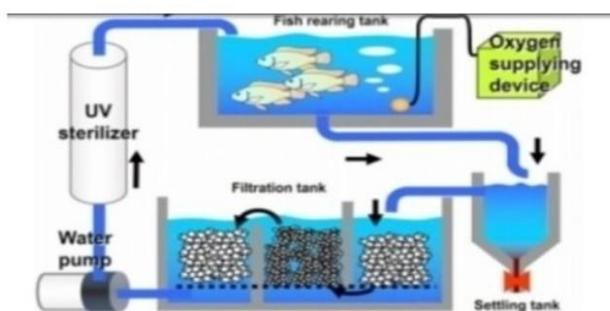
Figure 18 Schematic diagram of recirculating aquaculture system (Endo 2018).
